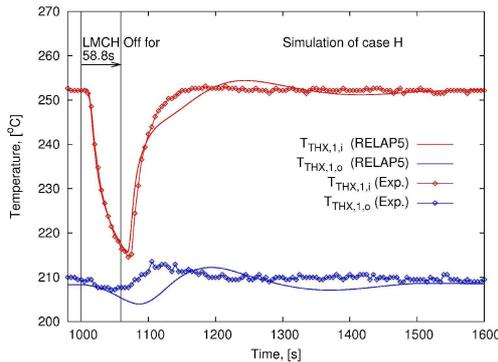
FIGURE N°6 : Comparison of experimental and calculated temperatures for an unprotected trip.
