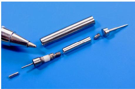
FIGURE N° 9: Micro fission chambers.
