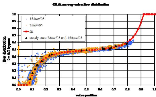
FIGURE N°3: Oil three way valve characteristics.
