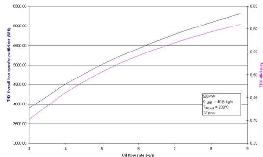
FIGURE N° 4 : Influence of oil flow-rate on Heat transfer coefficient
